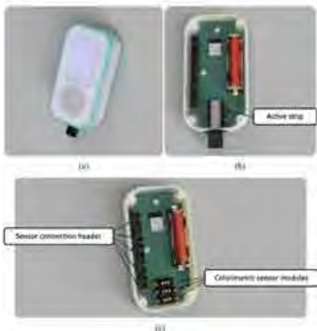
Figure: SAD, Salivary Analytical Device render. a) general view of the device prototype, b) housing arrangement of a commercial strip, c) arrangement of sensor connection header and connector colorimetric sensor modules.
